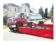
On December 29, 2011 Schuyler Hose Co. placed its new tanker in full service. TA-574 is a 2011 E-One Water Master Vacuum Tanker on an International 7400 chassis with seating for a crew of two. The tanker is equipped with a 1250 gpm Hale Pump, a Vacuum Pump and 3500 gallon aluminum water tank.
